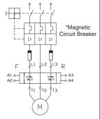
Overload protection of the motor is easily achieved by installing a manual thermal magnetic circuit breaker on the supply side of the motor.
